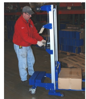
Lower the forks until the load is a few inches above the adjustable leg (shown by arrow in photo above).
