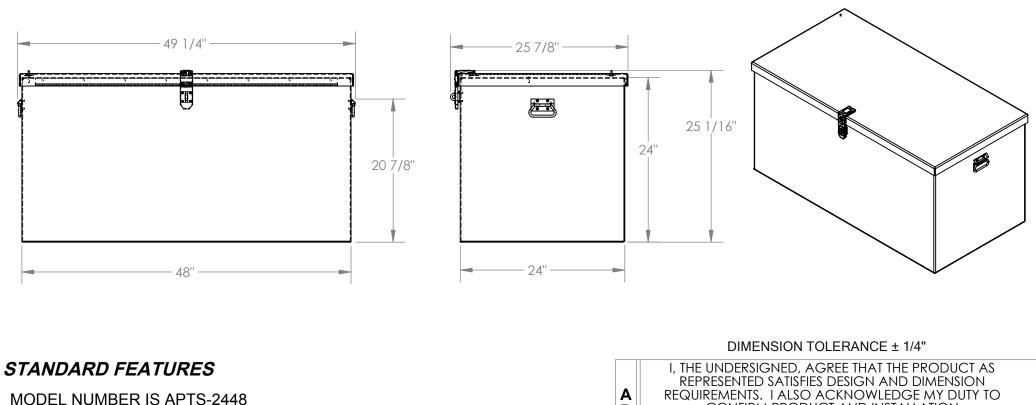
OVERALL WIDTH IS 49 1/4" **USABLE WIDTH IS 48"** OVERALL DEPTH IS 25 7/8" **USABLE DEPTH IS 24" OVERALL HEIGHT IS 25 1/16" USABLE HEIGHT IS 24"** MAX CAPACITY IS 2500 LBS.
