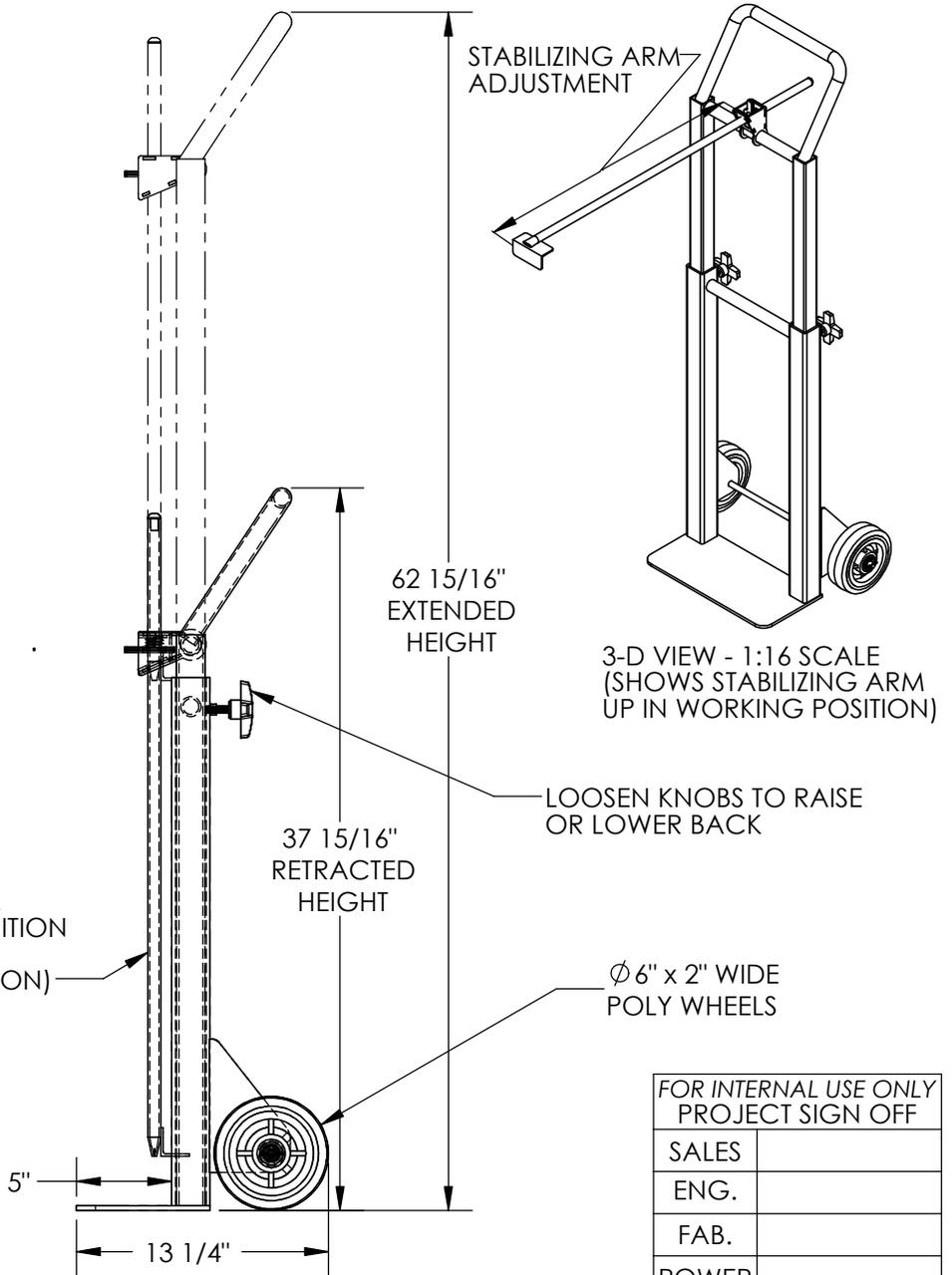
STABILIZING ARM IN STORAGE POSITION (SWINGS UP TO WORKING POSITION)
