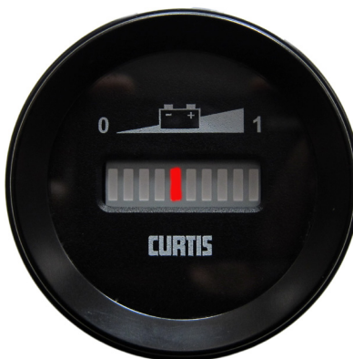
Insufficient. Battery charging is required but not urgent.
